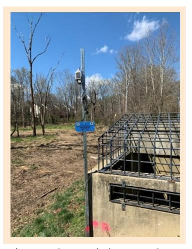
Long term real-time water level monitoring at the County's dam sites will help identify potential clogging and other issues to assist preventive maintenance.
