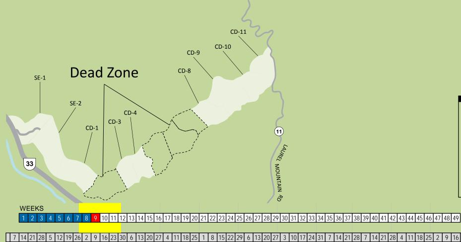
Scale: 1 mile Completed During Current Week Clearing and Grubbing Roadway Pad Site Excavation Foundation and Crane Pad Base/Mid Grouted WTG Mechanical Completion
