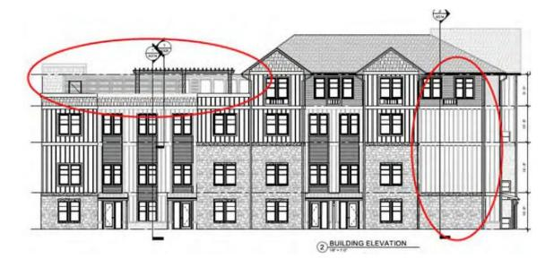
Finally, Flournoy proposes to add doors to the north façade (facing Dawson Farm Road) for additional access to the main patio, change the window style for two windows, and remove three windows on the third floor to align with the design of the corner unit. Exhibit 58 (shown on the next page).
