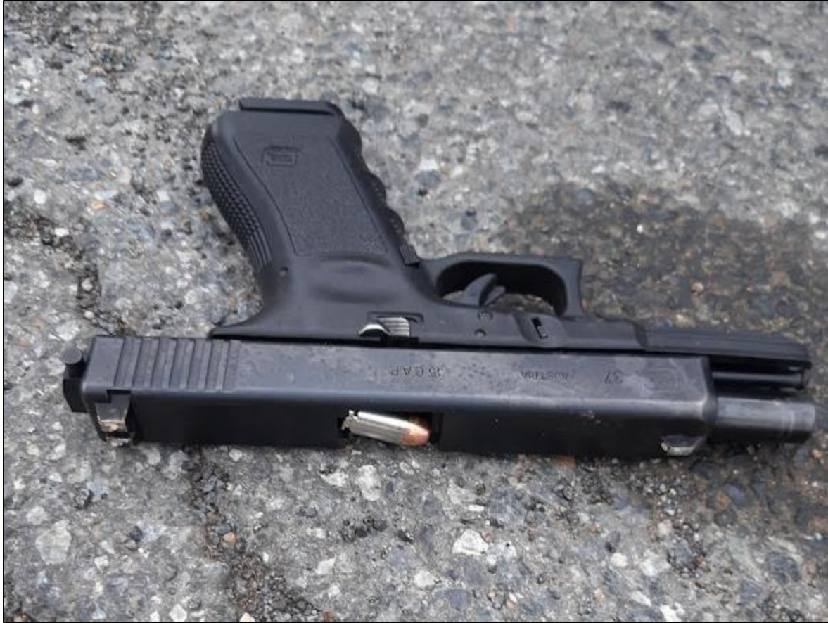
Image 3. Photograph of the Glock model 37 .45 GAP caliber pistol recovered from the crime scene, showing a live round of ammunition jammed between the frame and slide of the gun.
