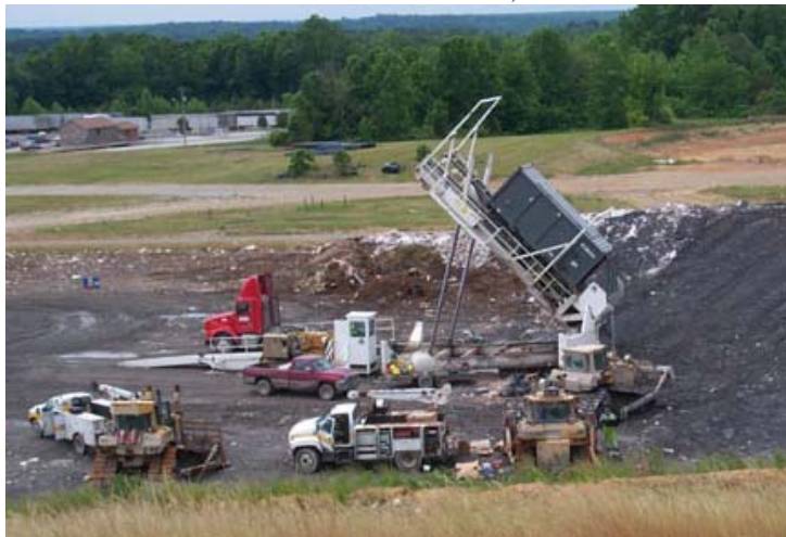
Montgomery County RRF Ash Being Dumped In The Montgomery- County Dedicated Landfill Cell At The Waste Management, Inc. Landfill in Brunswick, VA.
