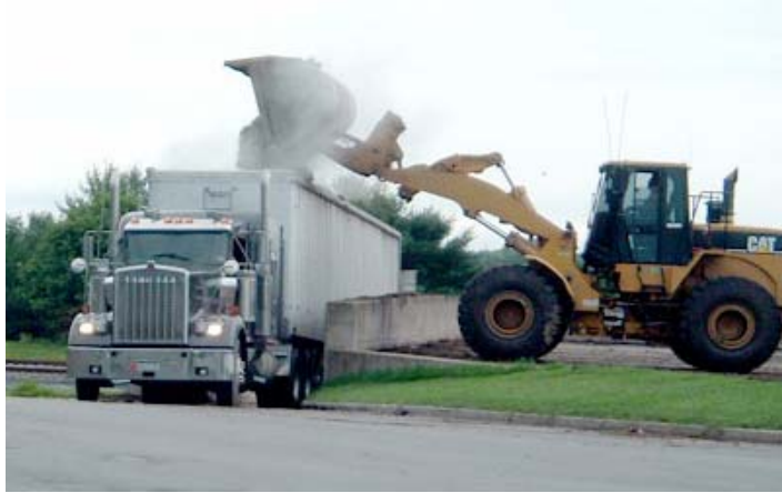
Ground Yard Waste Being Loaded At the Transfer Station Into A Walking-Floor Transfer Trailer for Transport to the Compost Facility
