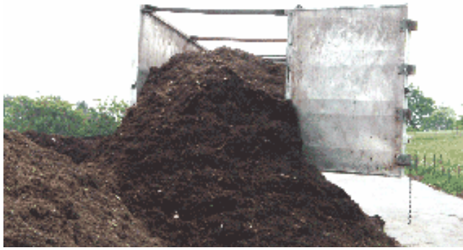
Special Yard Waste Rail Off-Loading at the Compost Facility Using a Tipping Chassis
