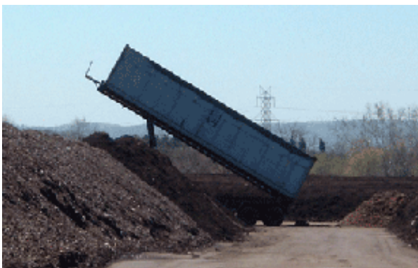
Special Yard Waste Rail Off-Loading at the Compost Facility Using a Tipping Chassis
