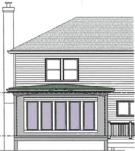
3 PROPOSED REAR ELEVATION (HIP ROOF WITH LOW SLOPE METAL ROOF) SCALE: \frac{1}{4} " = 1'-0"
