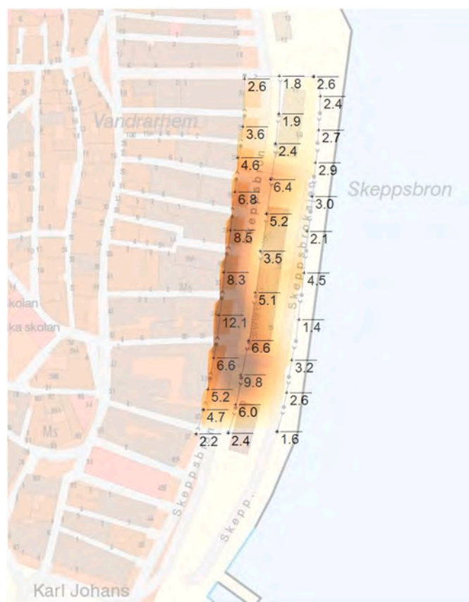
Fig. 2. Spatial distribution of the radiofrequency field (values in V m^{-1} ) at Skeppsbron street, based on spatial average of a given quadrat cell; hotspots are displayed in darker red where pedestrians are exposed at close range or rays overlap from several mobile phone base station antennas; the investigated area measures about 250 m North to South; map by Lantmäteriet, Sweden. (For interpretation of the references to colour in this figure legend, the reader is referred to the Web version of this article.)
