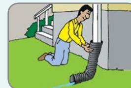
Cap outlet with old nylon stocking and seal downspout connections. If possible, replace corrugated with smooth PVC.
