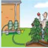
Determine the size of the runoff drainage area for a particular downspout, and calculate the size of the rain barrel(s) you will need.
