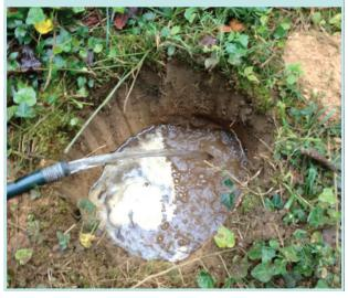
Check the hole periodically. When it is empty, record the time. Calculate how long it took to drain.
