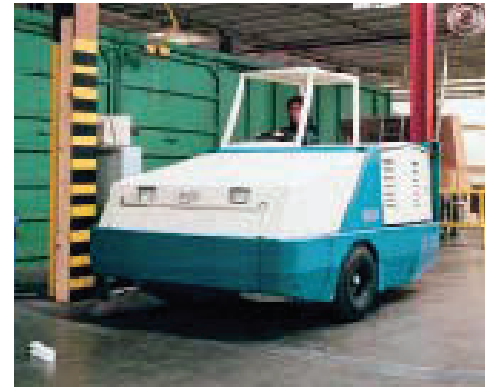
This rugged machine practically pampers its operators with an energy absorbing seat, tilt steering wheel, power steering, and an adjustable drive pedal.
