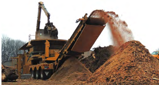
Figure 3-7. Tub Grinder. Photo courtesy of BioCycle CONNECT LLC.
