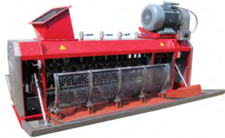
Figure 3-8. Mechanical Depackager. Photo courtesy of Dupps Mavitec.
