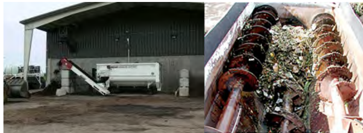
Figure 3-9. Mechanical Mixers. Photo courtesy of Coker Composting and Consulting.
