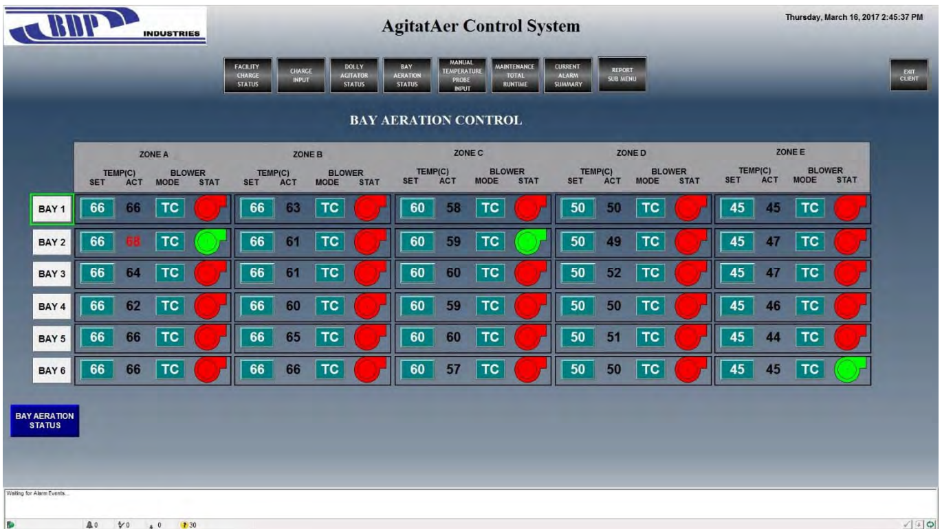
Photo 16 – Sample Blower Control Screen
