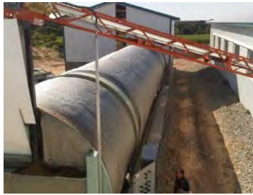
Figure 3-3. Rotating Drum Composting. Photo of XACT Systems, Trenton, Ontario, Canada.
