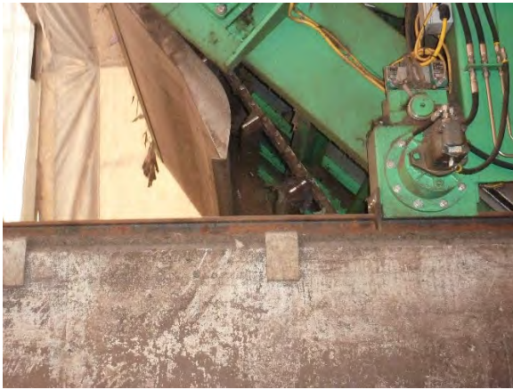
Photo 6 - Capacity Optimization Gate (COG) in closed position near bay discharge
