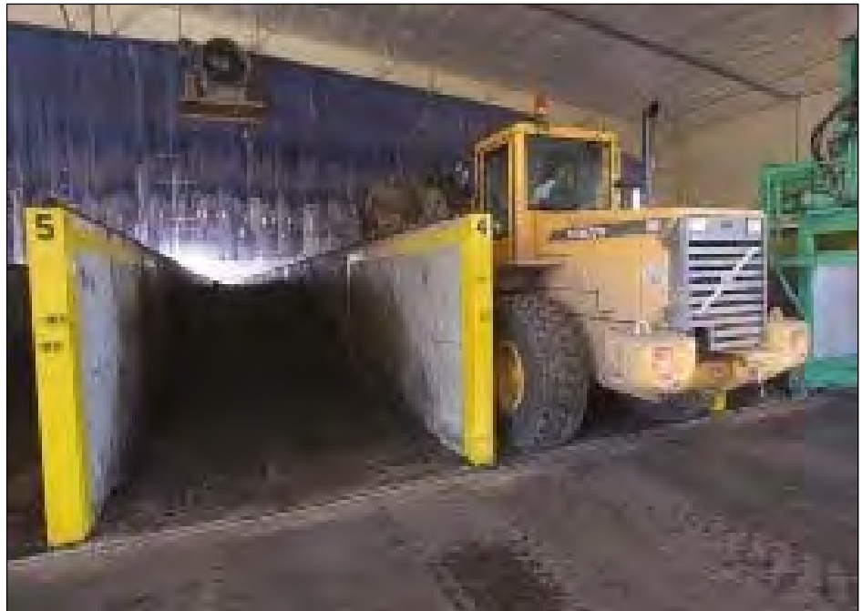
Photo 2 - Front End Loader “Charging” Bays
