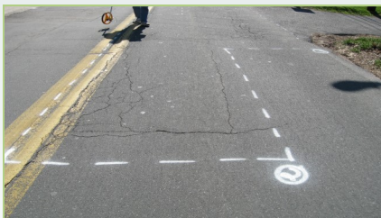
Typical survey paint markings
