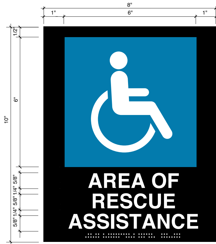
PL10 AREA OF RESCUE ASSISTANCE SIGN
