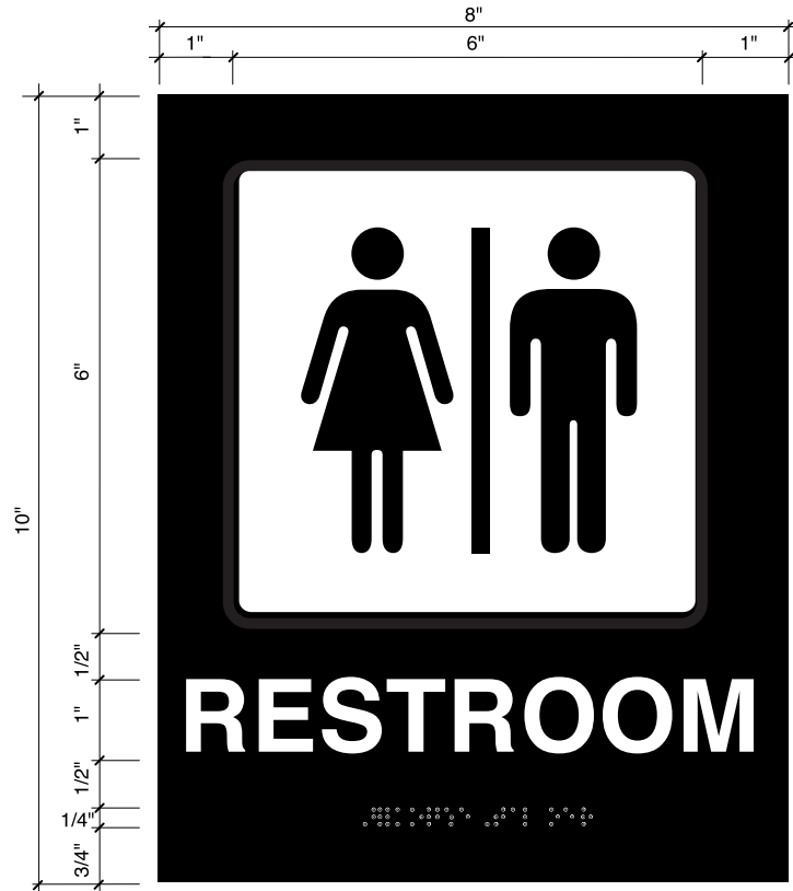
CO3 - RESTROOM PLAQUE - TYPICAL SCALE: 3/8"=1"
