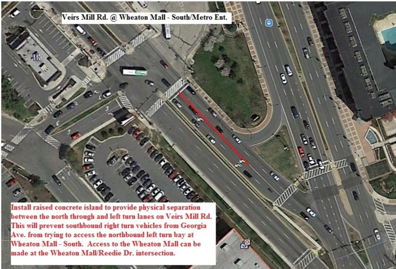
**Figure 2: Veirs Mill Road at Wheaton Plaza South/Metro Entrance - proposed channelization - northbound left turn bay.**
