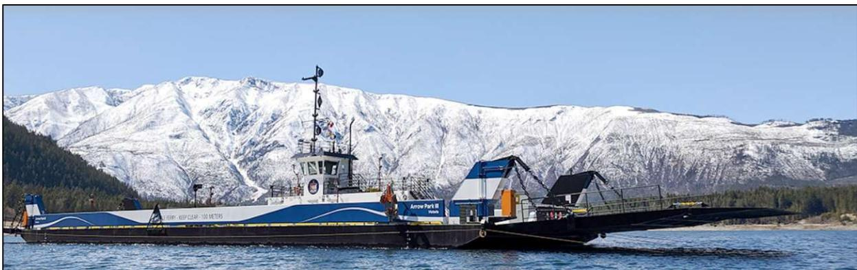
Figure 4-19: Another Example of Ferry with a Boat Based Loading Ramp
