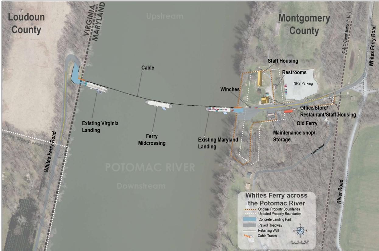
The Maryland side serves as the base of operations for the Ferry service and has office space, staff housing, washrooms, a store, fuel storage, and a maintenance shed. The Virginia side has no additional facilities beyond the loading ramp and the cable winch.
