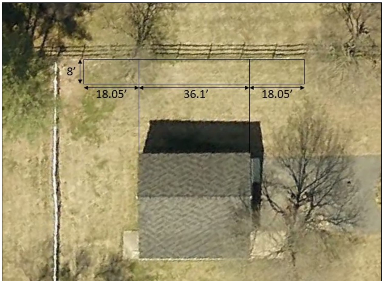
Figure 9. Length of screening required along rear property line shown on 2019 aerial image. The screening must be the length of the barn plus 50% of this length on either side. The screening is required to be eight or twelve feet wide, depending on the selected screening option.
