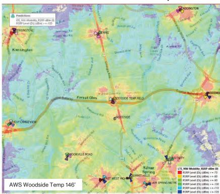
Note: The Woodside site (as well as the temp site) is not only a coverage site, but more importantly a "capacity" site. Without the Woodside site, "capacity" of the surrounding cell sites would suffer with overall wireless service in the broader area adversely impacted.
