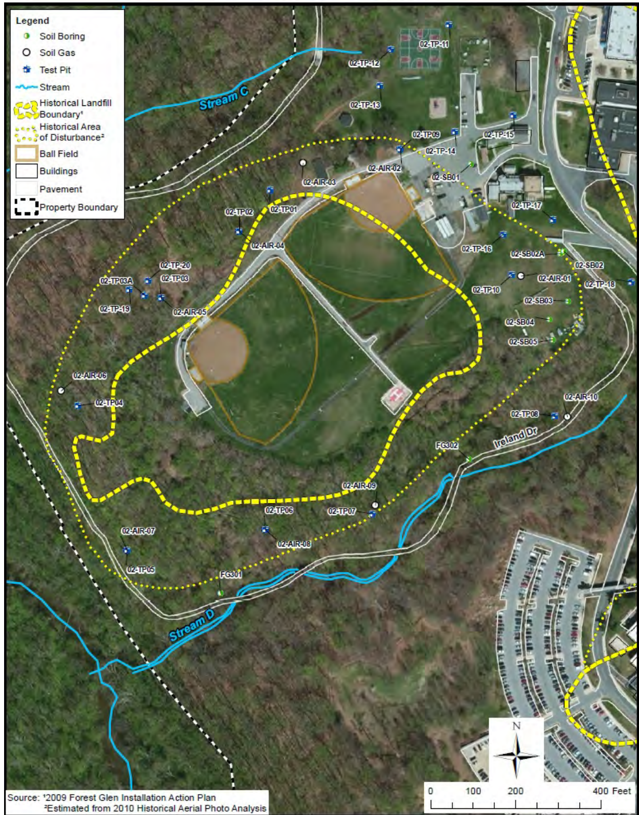
Figure 4-5: Subsurface soil sample locations
