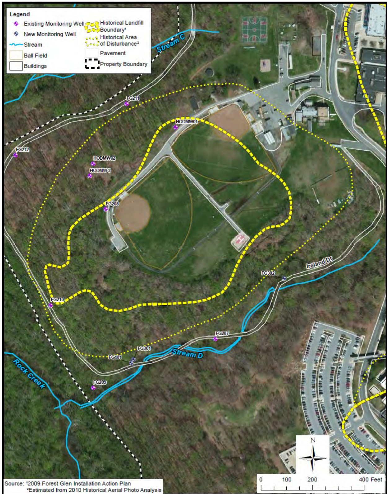
Figure 4-7: Groundwater monitoring well locations
