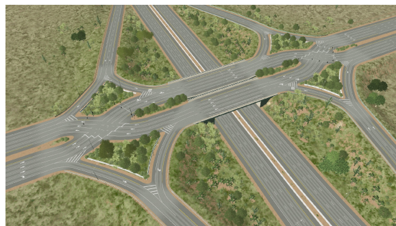
A diverging diamond interchange
