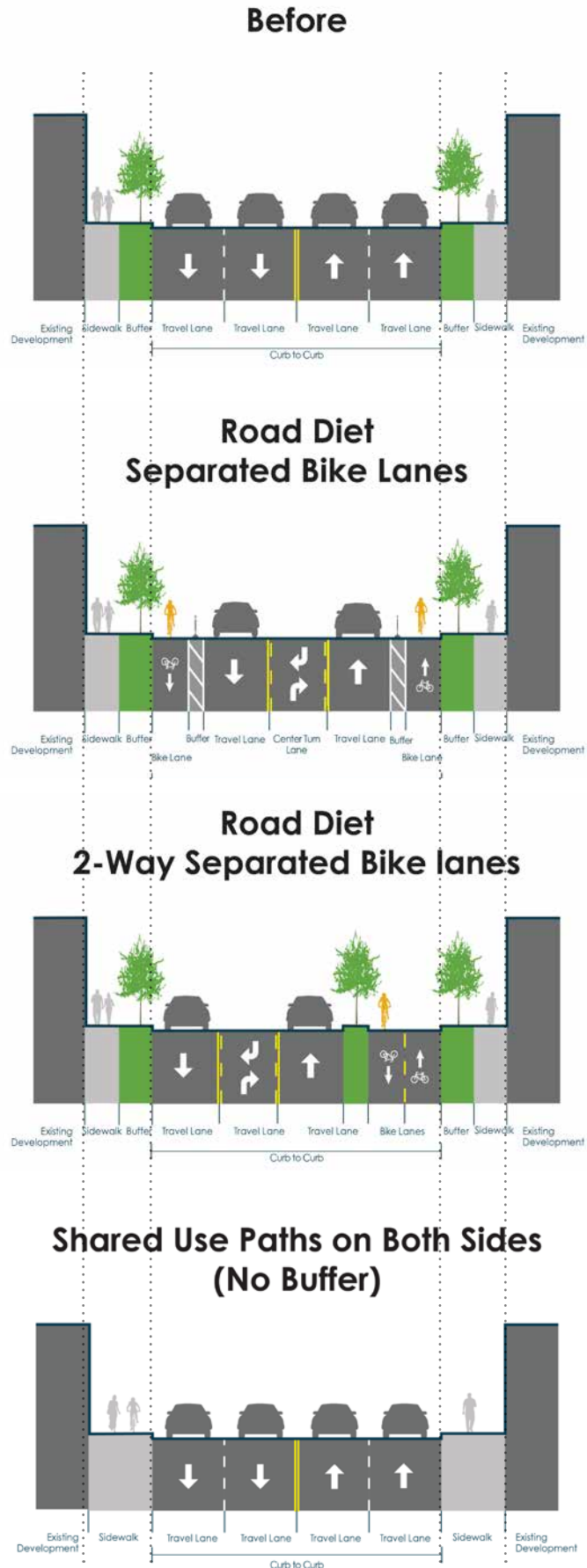
Figure 4.7: Example Street Cross Section to illustrate implementation of bicycle facilities without widening.
