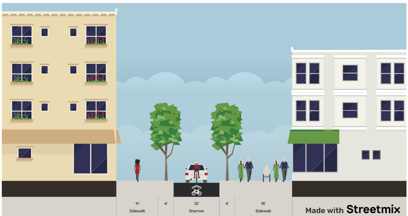
Figure 13: Alternative 2 Cross Section (Newell Street One-Way Westbound)
