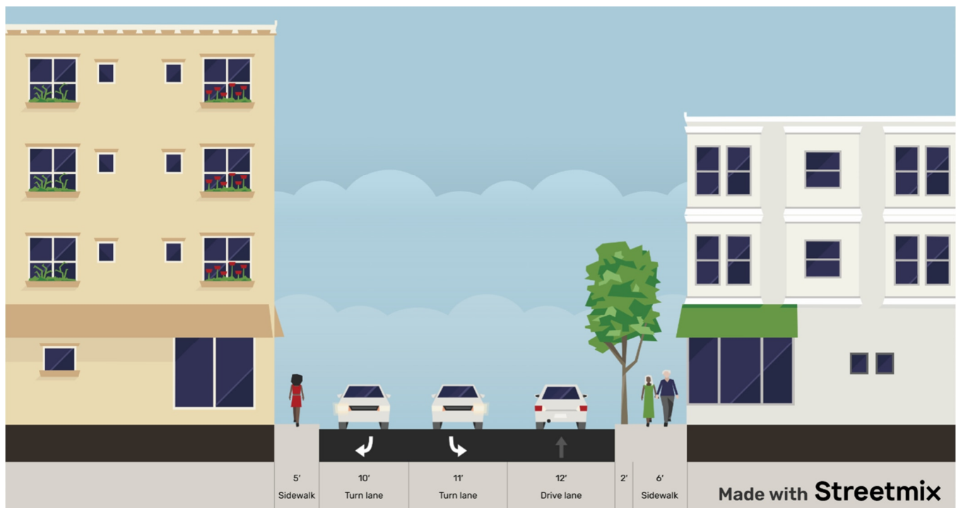
Figure 2: Existing Cross Section of Newell Street looking west
