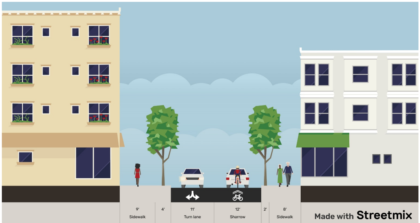
Figure 12: Alternative 1 Cross Section (Two-Way with Removal of Eastbound Right Lane)
