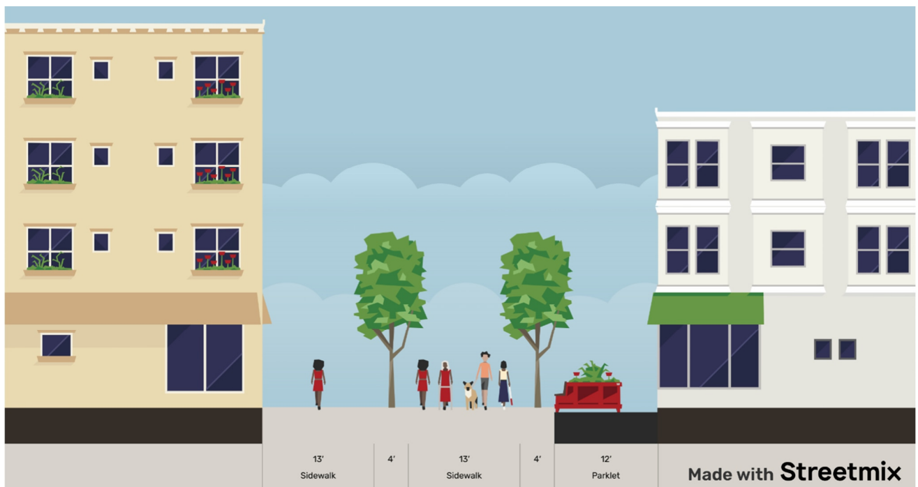
Figure 15: Alternative 4 Cross Section (Full Closure of Newell Street)
