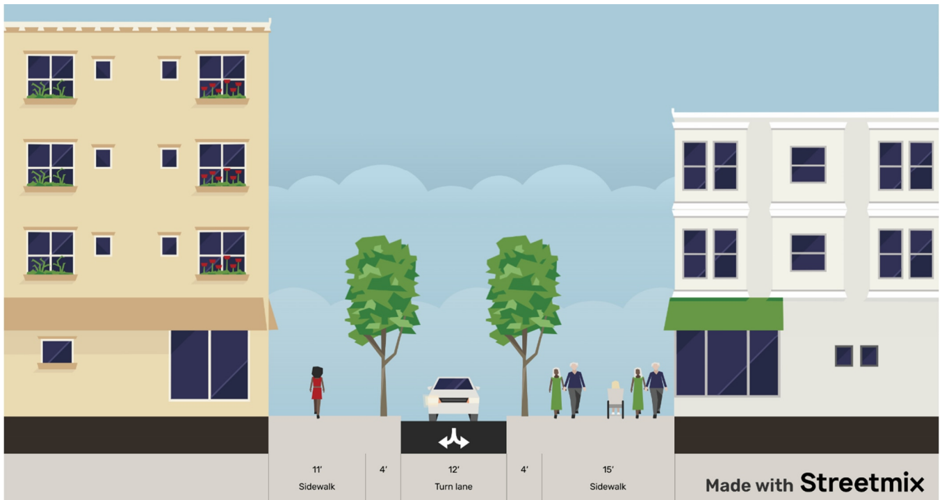
Figure 14: Alternative 3 Cross Section (Newell Street One-Way Eastbound)
