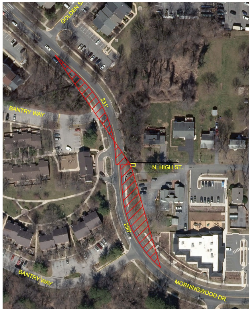
Figure 5-1: North High Street Intersection Required Sight Distance
