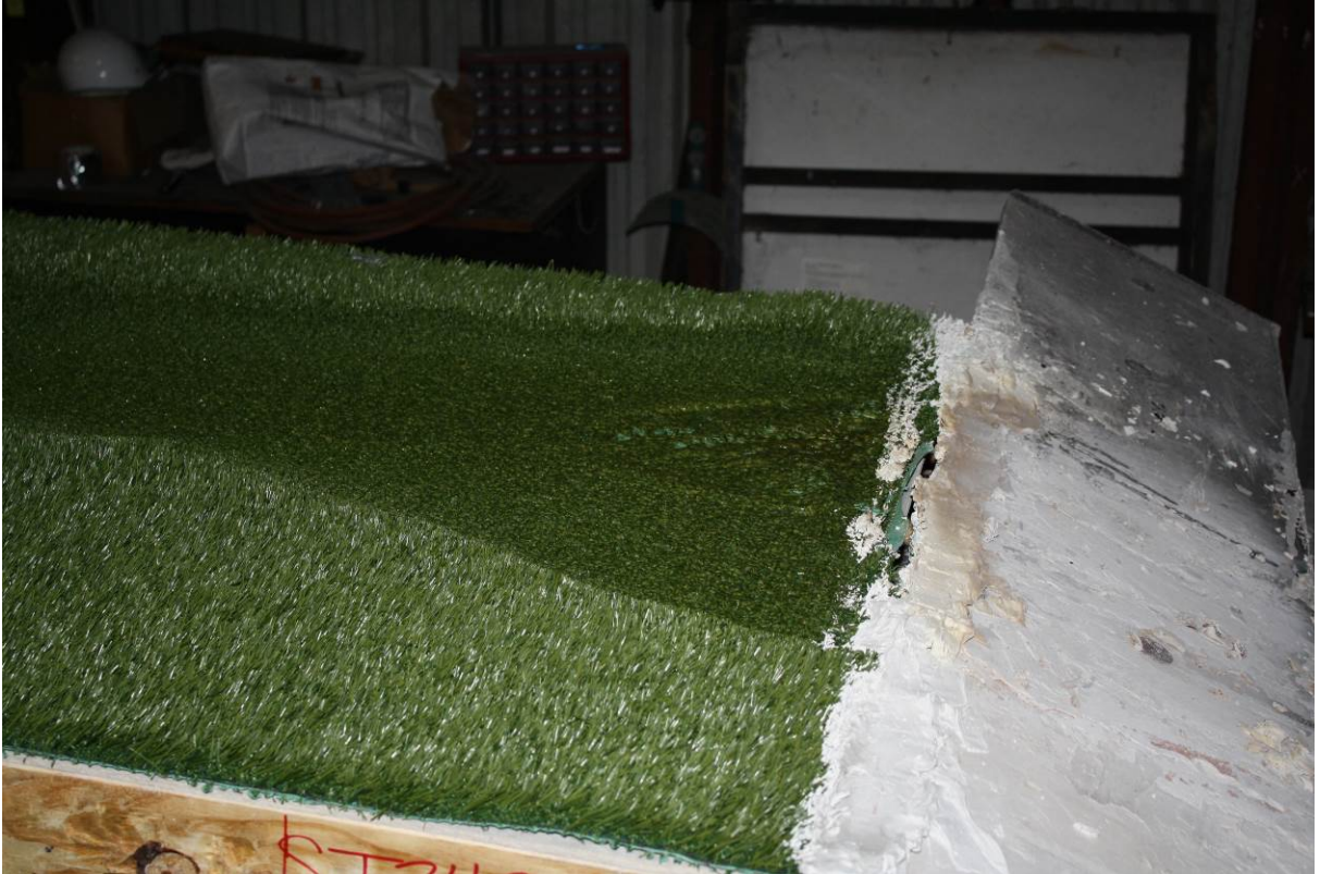
Figure B-2. SoF Test #1. Sample after flame exposure.
