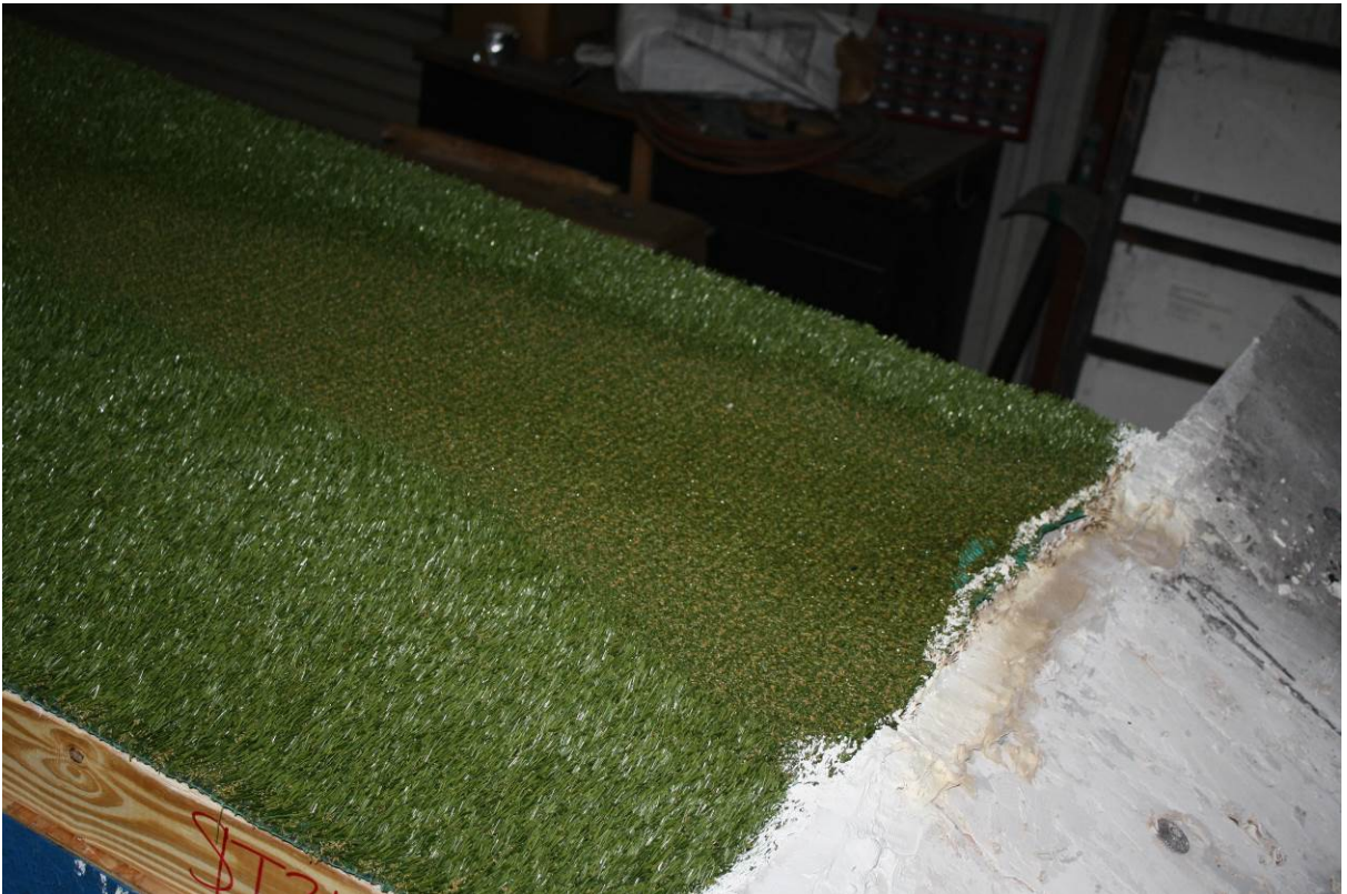
Figure B-4. SoF Test #2. Sample after fire exposure.
