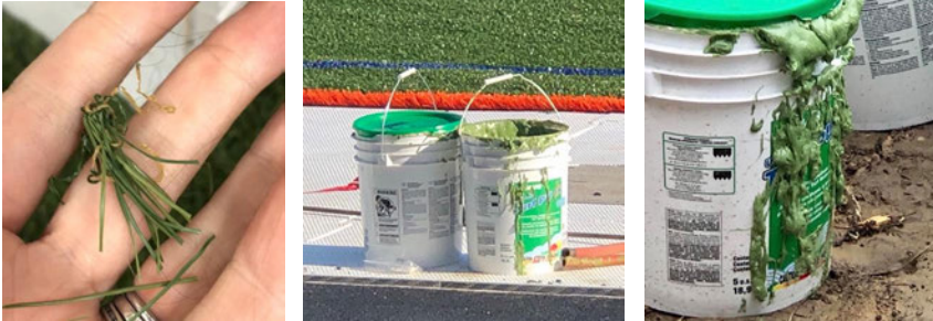
Pieces of SynLawn coming loose at the Lawn exhibit at the National Building Museum, turf glue used in artificial turf installations.
