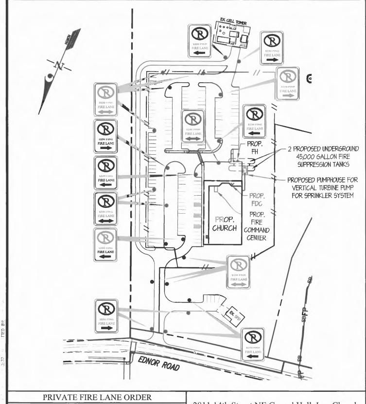
PROPOSED "NO PARKING-FIRE LANE" SIGN PROPOSED YELLOW FIRE LANE CURB PAINTING PROPOSED PAINTED RED FIRE LANE STRIPING ON PAVEMENT. (WHERE THERE IS NO CURB, AS SHOWN ON THE PLAN ONLY).
