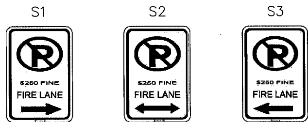
FIRE LANE SIGNS
