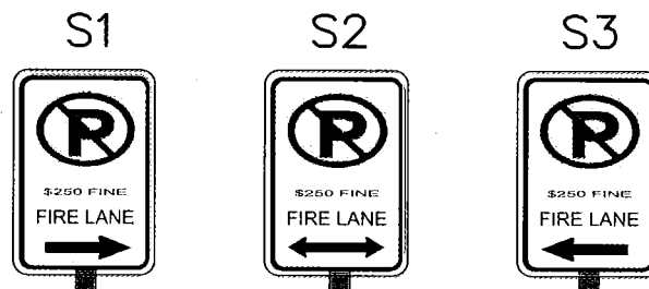
FIRE LANE SIGNS
