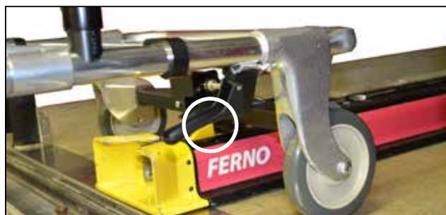
Figure 28 - Loading Post Past Safety Stop
