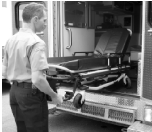
Figure 45: Pull the Cot out of the Vehicle
