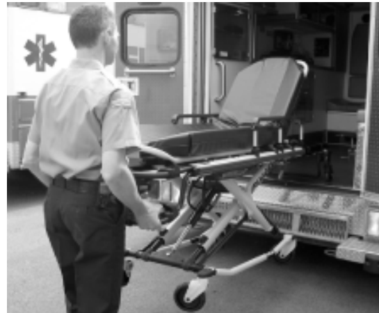
Figure 46: Pull the Manual Back-up Release Handle and Roll the Cot out of the Vehicle
