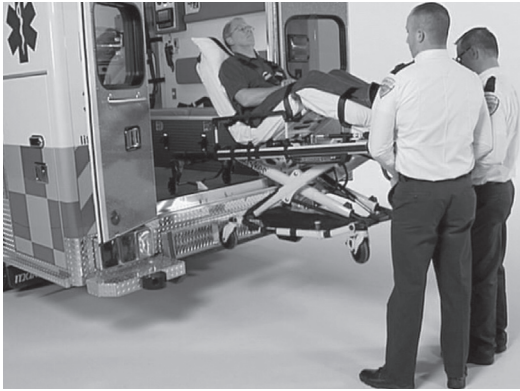
Figure 21: 2 Operators (Foot End) - One Pressing the Retract Button
