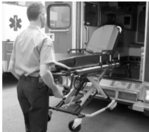
Figure 35: Roll the Cot out of the Vehicle
