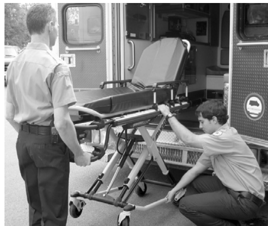
Figure 38: 2 Operators - One Lifting Base
