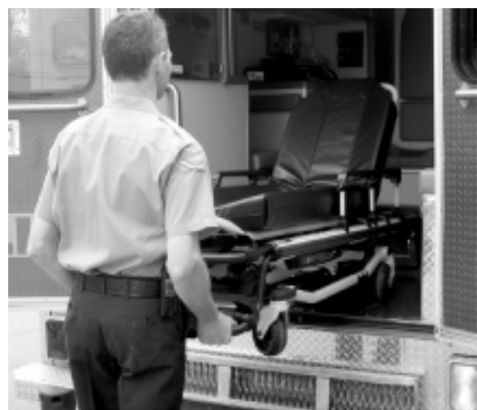
Figure 39: Push the Cot Into the Vehicle
