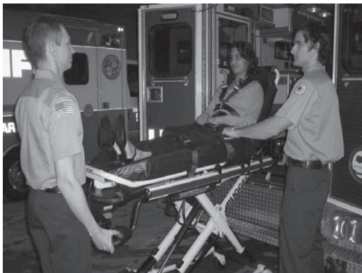
Figure 23: 2 Operators (Foot End and Side) - One Pressing the Retract Button
