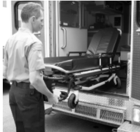
Figure 33: Pull the Cot out of the Vehicle
