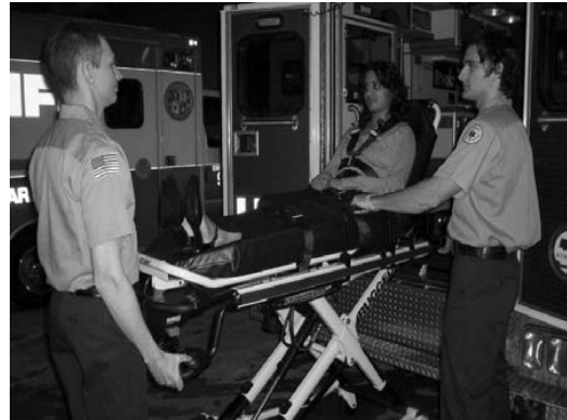
Figure 43: 2 Operators (Foot End and Side) - One Pulling the Manual Back-up Release Handle
