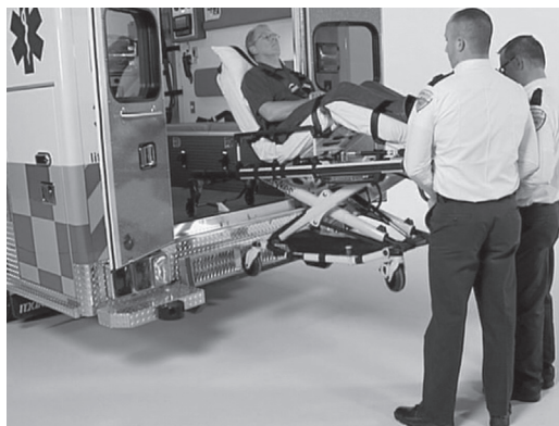
Figure 29: 2 Operators (Foot End) - One Pressing the Extend Button
