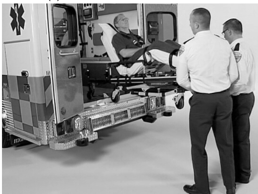
Figure 28: 2 Operators (Foot End) Unloading the Cot
