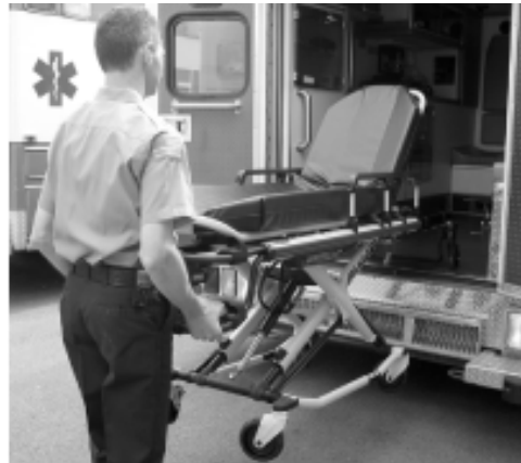
Figure 25: Load Wheels on the Vehicle Floor
