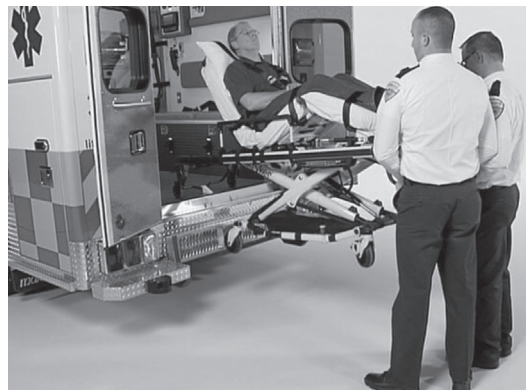
Figure 41: 2 Operators (Foot End) - One Pulling the Manual Back-up Release Handle
