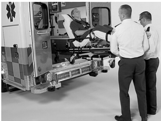
Figure 40: 2 Operators (Foot End) Unloading the Cot
