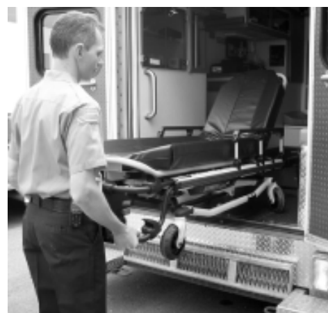
Figure 27: Push the Cot into the Vehicle
