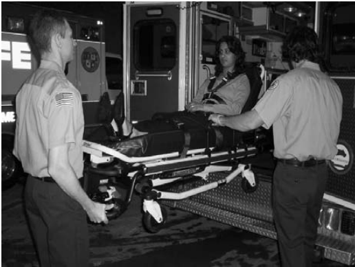
Figure 30: 2 Operators (Foot End and Side) Unloading the Cot
