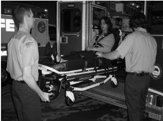
Figure 42: 2 Operators (Foot End and Side) Unloading the Cot
