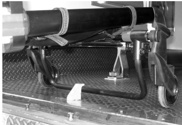
Figure 20: Safety Bar Engaging Safety Hook
