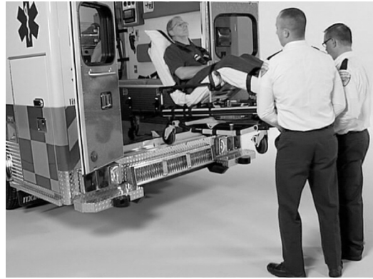
Figure 22: 2 Operators (Foot End) Loading the Cot
