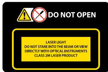
Do Not Open/Laser Notice Location: Controller Housing
