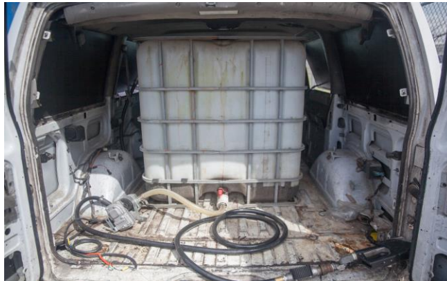
Plastic container was intended for soap or other non-flammable liquid. Note the hoses and wires leading to the transfer pump.
