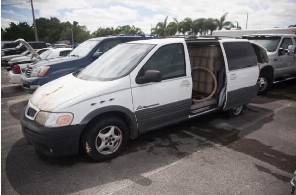
Dark or painted rear windows to conceal bladder tank
