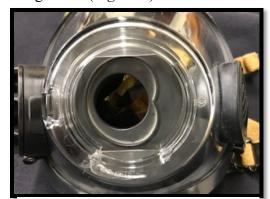
Figure 1 Lens Crack Location
