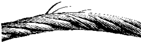
Wire Rope Fatigue Failure
