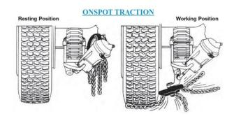
A primary benefit of this chain system is that the driver may engage and disengage it as roadway conditions change without leaving or stopping the apparatus. An electric switch mounted in the cab provides 12 volts to an air solenoid mounted on the vehicle's frame rail. Compressed air to the solenoid is supplied from either the vehicle's onboard air system or a 12-volt compressed air kit.
