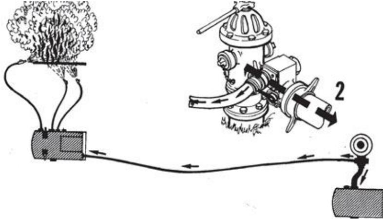
4. Connect a supply line from a discharge on the Supply Engine to the intake side of the Humat Valve.
