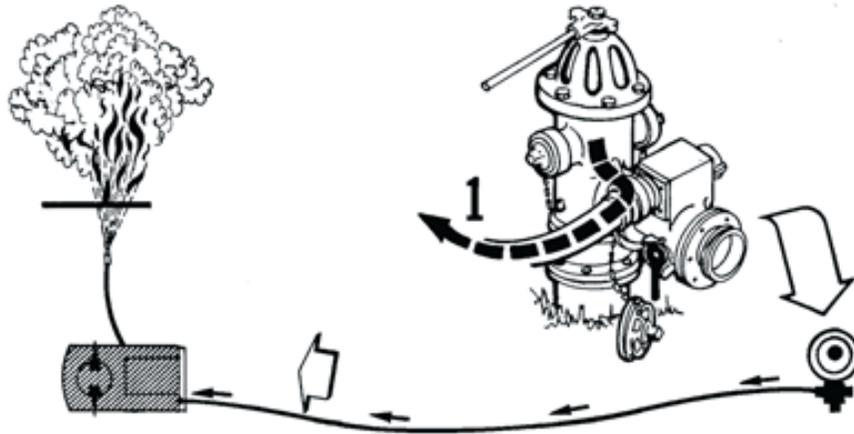
2. After ensuring the Attack Engine is ready for water, charge the hydrant to get an initial water supply to the Attack Engine.
