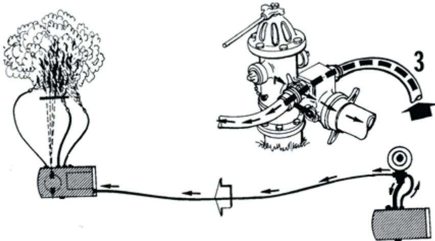
8. Once pressure from incoming supply line exceeds the hydrant pressure an internal clapper valve in the Humat Valve will close.
