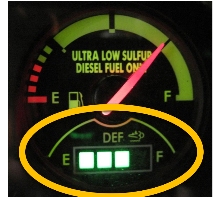
DEF Tank gauge located below fuel gauge on dash.
