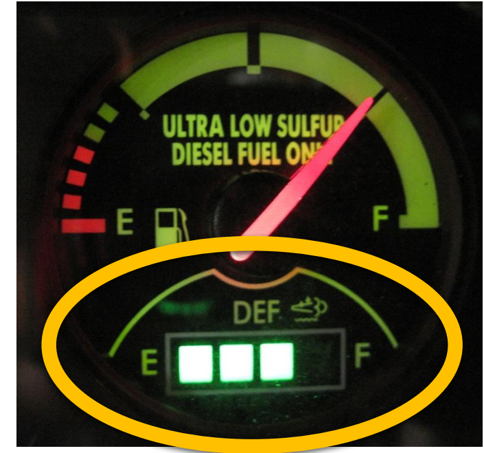
DEF Tank gauge located below fuel gauge on dash.
