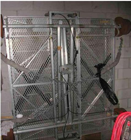
This is what an ETEC cart will look like in the stored position. Note: The cart is locked in position with a chain and padlock. (Disregard the trash bag tied to the bottom of the cart. If you run across something like this in the field you will just have to remove it from the cart before using it.)
