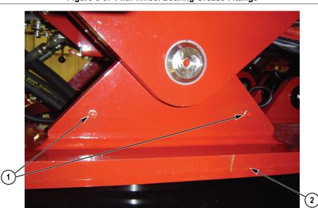
Figure 6-3: Fifth Wheel Bearing Grease Fittings
