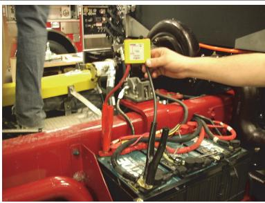
Figure 6-16: Connecting the Anti-Zap Device
