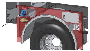
The Diesel Exhaust Fluid reservoir is typically located in the driver's side rear wheel fender behind the forward air bottle storage door. The DEF reservoir location on your apparatus may be different, depending on the rear body design. The reservoir has a blue cap and is accompanied by a DEF fluid only label.
