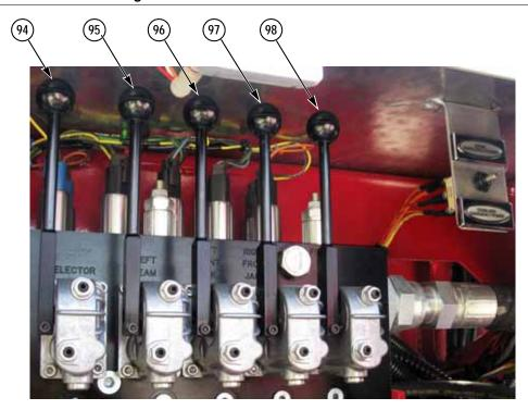
Figure 2-21: Manual Override Stabilizer Controls
