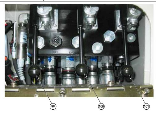
Figure 2-22: Manual Aerial Override Controls
