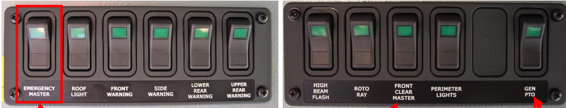
Warning Lights switch panels
