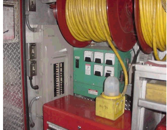
Typical Apparatus Based Electrical System
