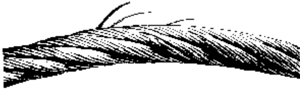
Wire Rope Fatigue Failure
