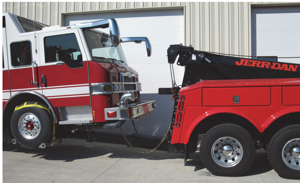
Figure 6-8: Underlift Device using Tire Lift Brackets
