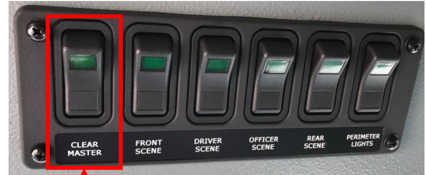
Scene light switch panel
