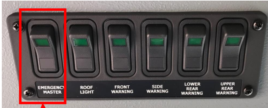
Warning light switch panel
