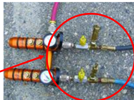
Relief valve placed at the airbag
