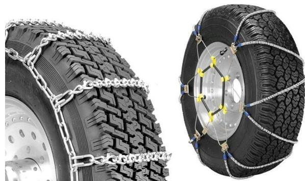
On tandem axle apparatus they should be applied to the drive axle wheels. Note: If chains are installed on a Pierce All-Steer, the all-steer functions must be disabled.
